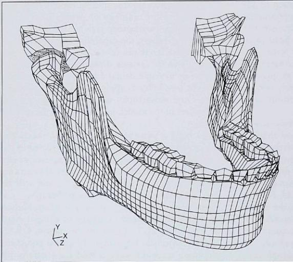
**Fig 2** FE model of the human mandible showing hidden line view of the discretized element mesh seen anterolaterally from the right side. Dental and articular restraints, as well as the muscle loads, have been omitted for clarity. Some elements of the right TMJ have been deleted to show the presence of a fibrocartilaginous pad (stippled) between the condyle and the temporal bone.
