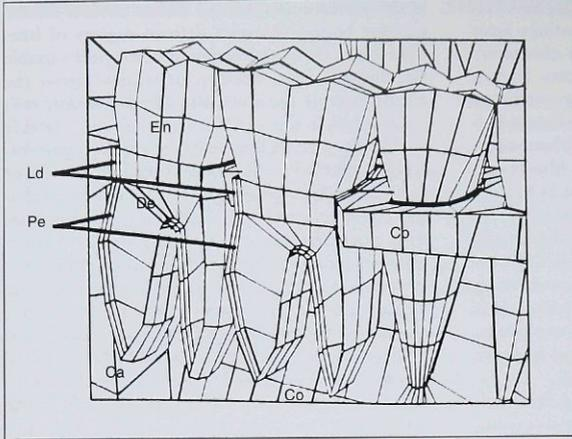
**Fig 1** FE model of the dentate human mandible; cut window of the right corpus displays the underlying tissue components. Many cancellous bone elements were deleted to reveal the dental roots. (Co = cortical bone; Ca = cancellous bone; En = enamel; De = dentin; Ld = lamina dura; Pe = periodontal ligament.)
