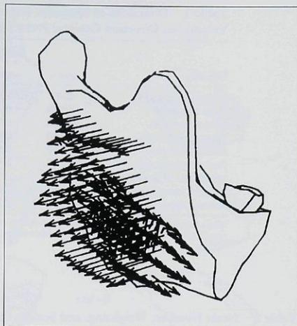
Fig 3 FE model of the human mandible showing right ramus with multiple parallel vectors simulating the masseter muscle loads. All vectors are graphically represented by their x, y, and z components and appear to be embedded in the model due to the nature of the display.
