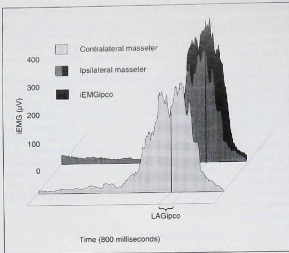
Fig 1 Rectified and smoothed EMG signals for one chewing cycle. The areas under the curve for the contralateral masseter EMG values are superimposed over the ipsilateral masseter EMG values. The variable iEMGipco represents the difference between these two areas. The time difference between the center of each area is represented by the variable LAGipco.
