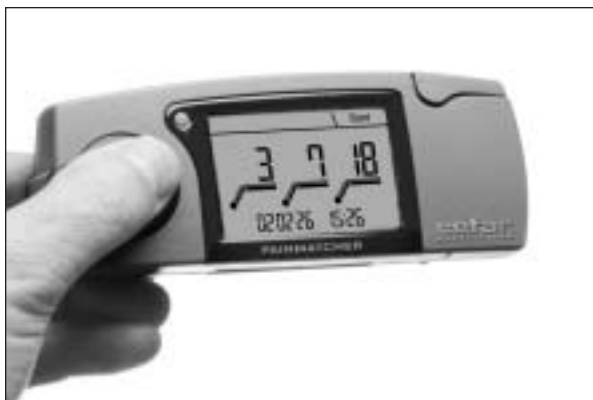
Fig 1 The pain-intensity matching device (score 0 to 60) consists of a unit for application of electricity to the thumb and index finger. The Painmatcher creates an eventually noxious stimulus by progressively increasing electrical intensity.
