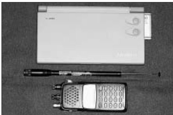
Fig 3 All components of the recording. From top to bottom: portable laptop computer with an A/D card, an antenna, and a receiver.
