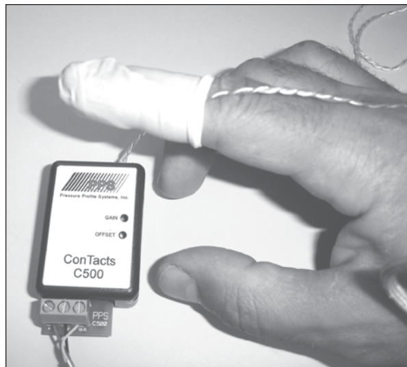
Fig 1 The sensor “ConTacts C-500” of the PAP attached to the index finger.
