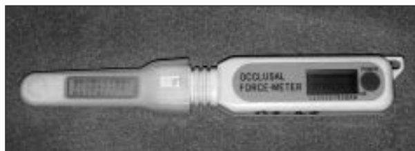
Fig 1 Bite force meter with disposable cover.
