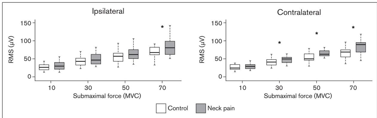
**Fig 4** Boxplots of the average normalized root mean square (RMS) values recorded from the ipsilateral and contralateral masseter muscles during unilateral jaw clenching at 10%, 30%, 50%, and 70% of the maximal voluntary contraction (MVC) in the control and patient groups. \* $P < .05$
