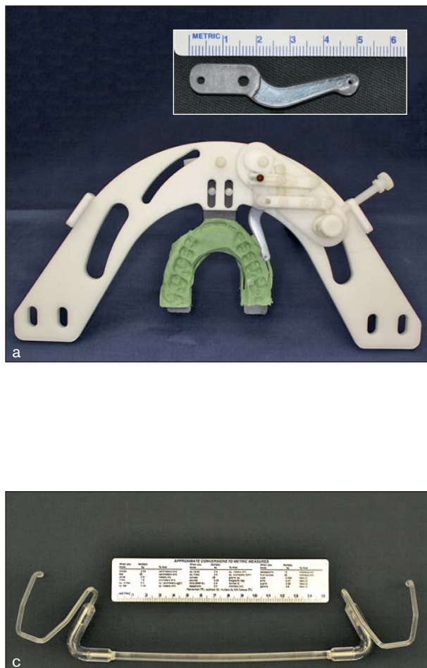
Fig 1 Stimulus device and dental chair-side use. (a) Top and (b) bottom views of the stimulus device fully assembled, and closer view of the intraoral probe (inset); (c) custom-made lip and cheek retractor (d) Subject rating dentoalveolar stimulation using COVAS in the dental chair. (Figs 1a to 1c reproduced from Moana-Filho et al 17 with permission from BioMed Central.)
